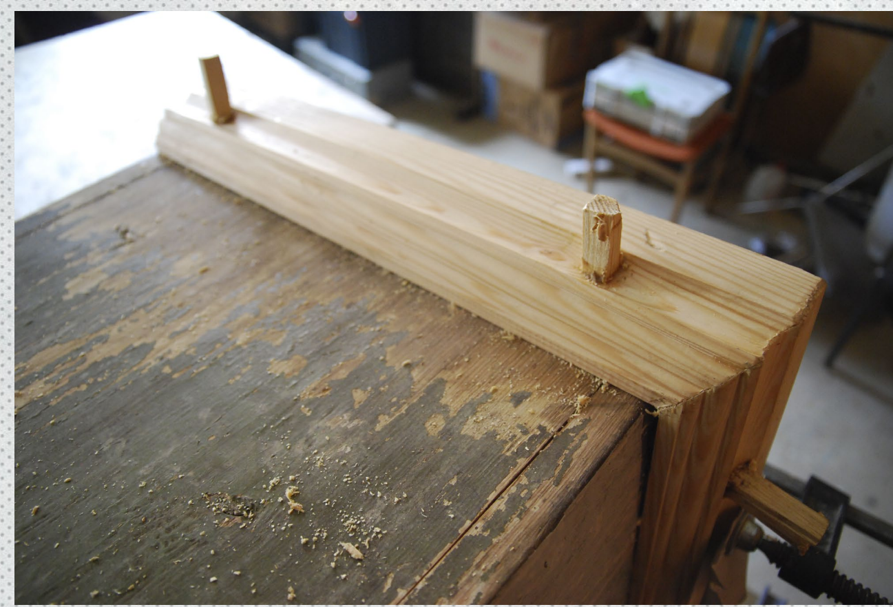
ill. 4. During restoration. Reconstruction of a stylized cornice on the bottom of the sideboard.
