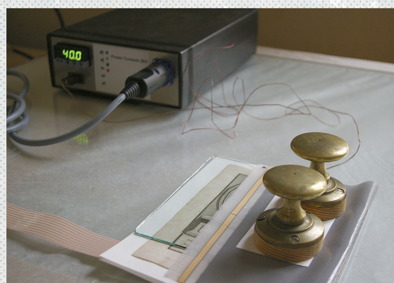
ill. 4 c. Folded extra flexible mat ensured heating from both sides.
