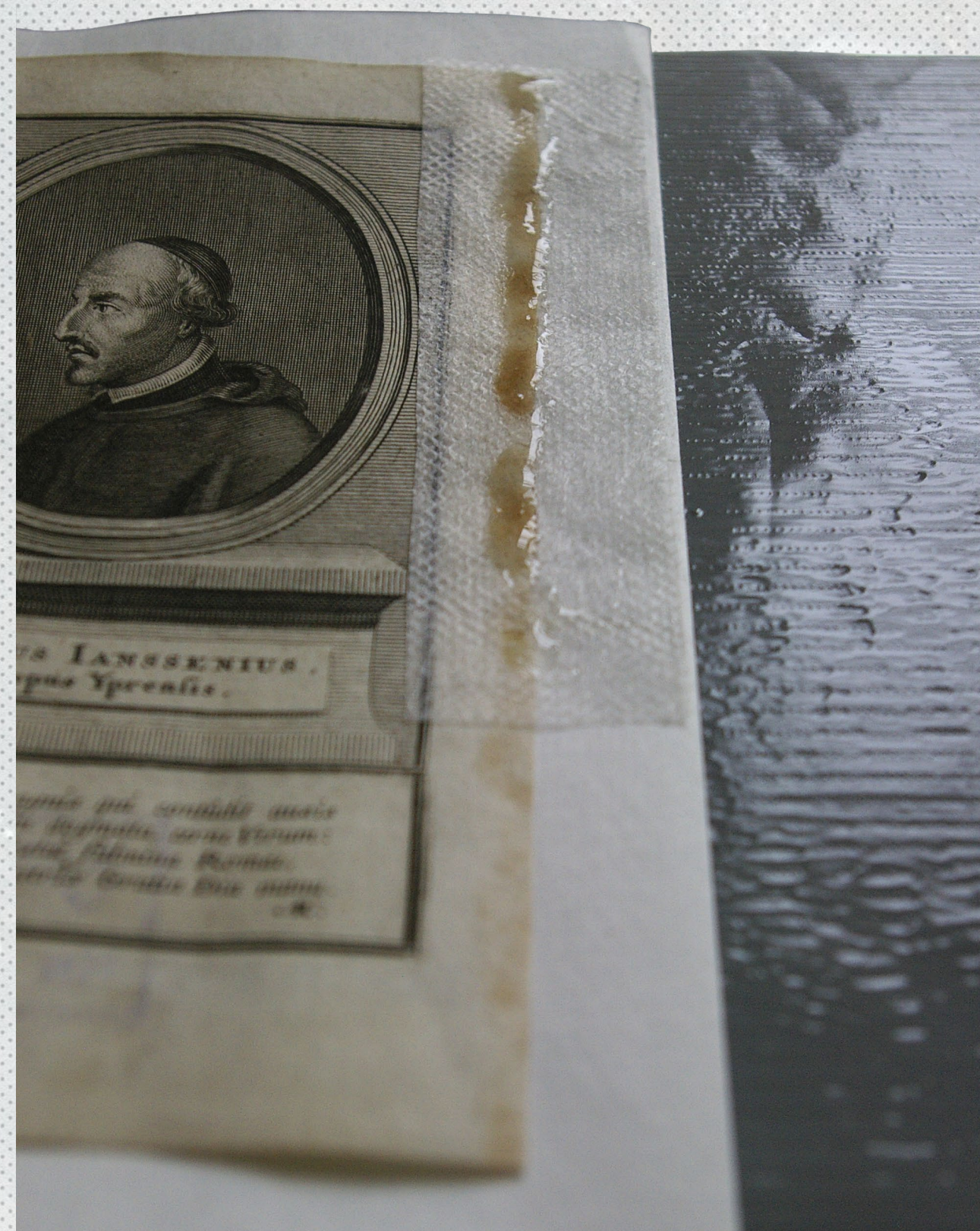
ill. 4 b. The enzyme Alcalase 2.4 L FG (Novozymes, Denmark) with Tylose MH300 as a carrier was pasted on paper through nonwoven polypropylene fabric. Conservator Rytė Šimaitė.
