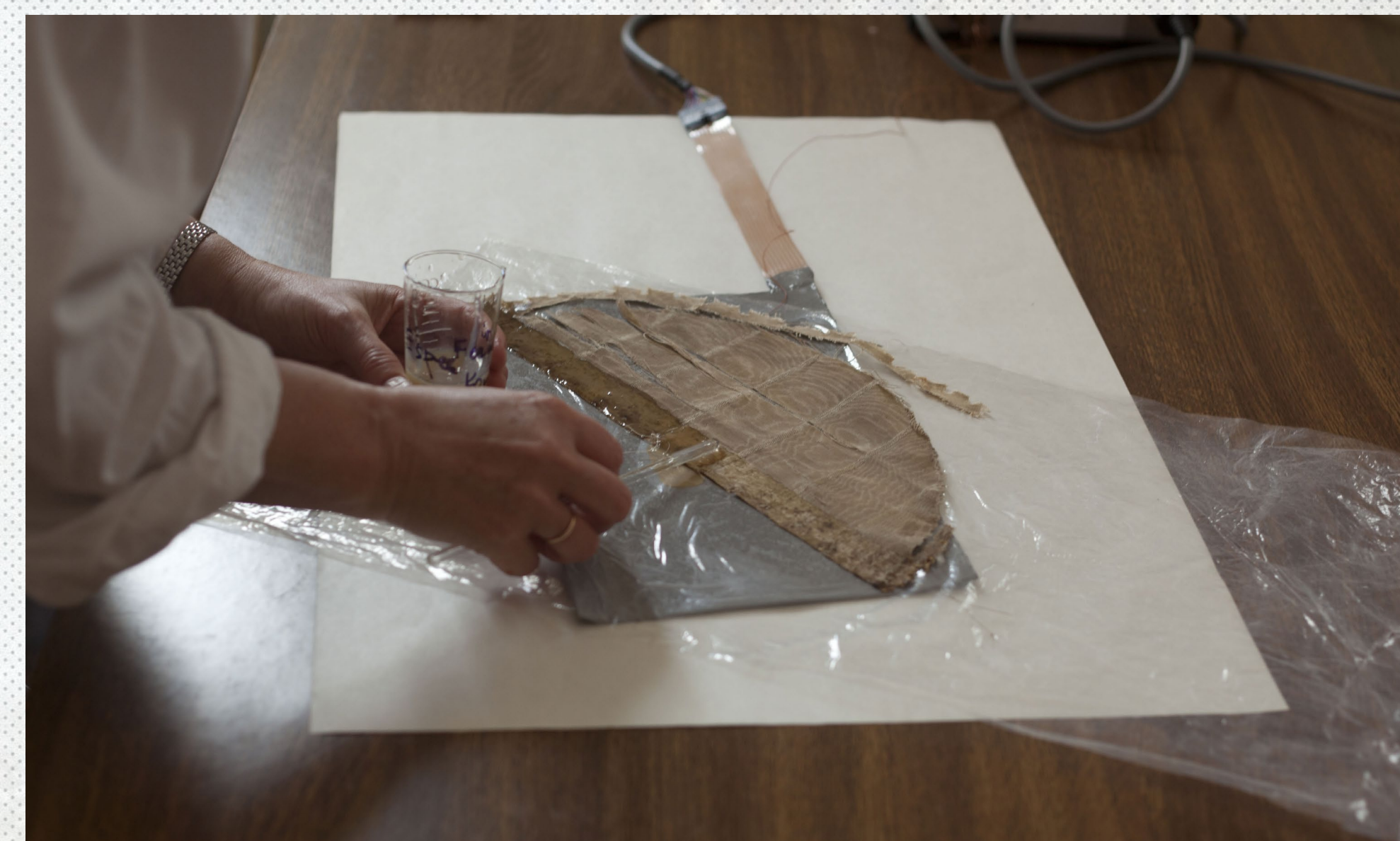
ill. 6 c. The mixture of enzymes Everlase 16L and Esperase 8.0L (Novozymes, Denmark) in Klucel E , done in sodium borate/potassium phosphate buffer (pH9), was applied on adhesive residues. Standard film heater and 40 °C was used. Conservator Danguolė Daugirdienė.
