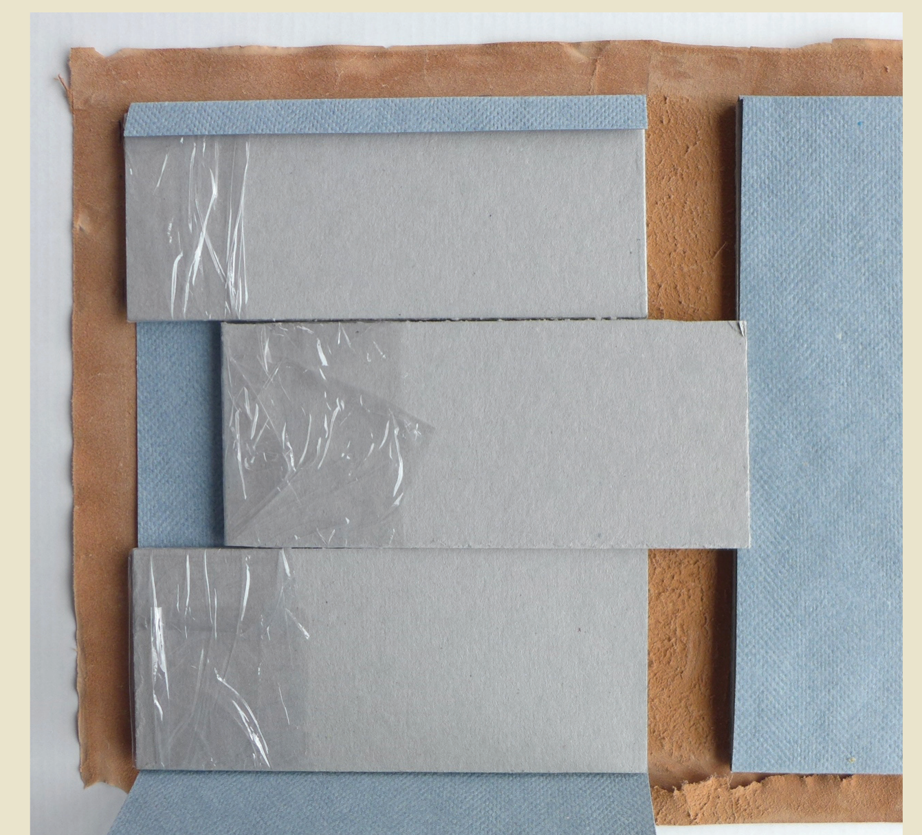
11. 3mm cardboard forming the mould is cut in 3 parts, the outer edges are covered with film.
