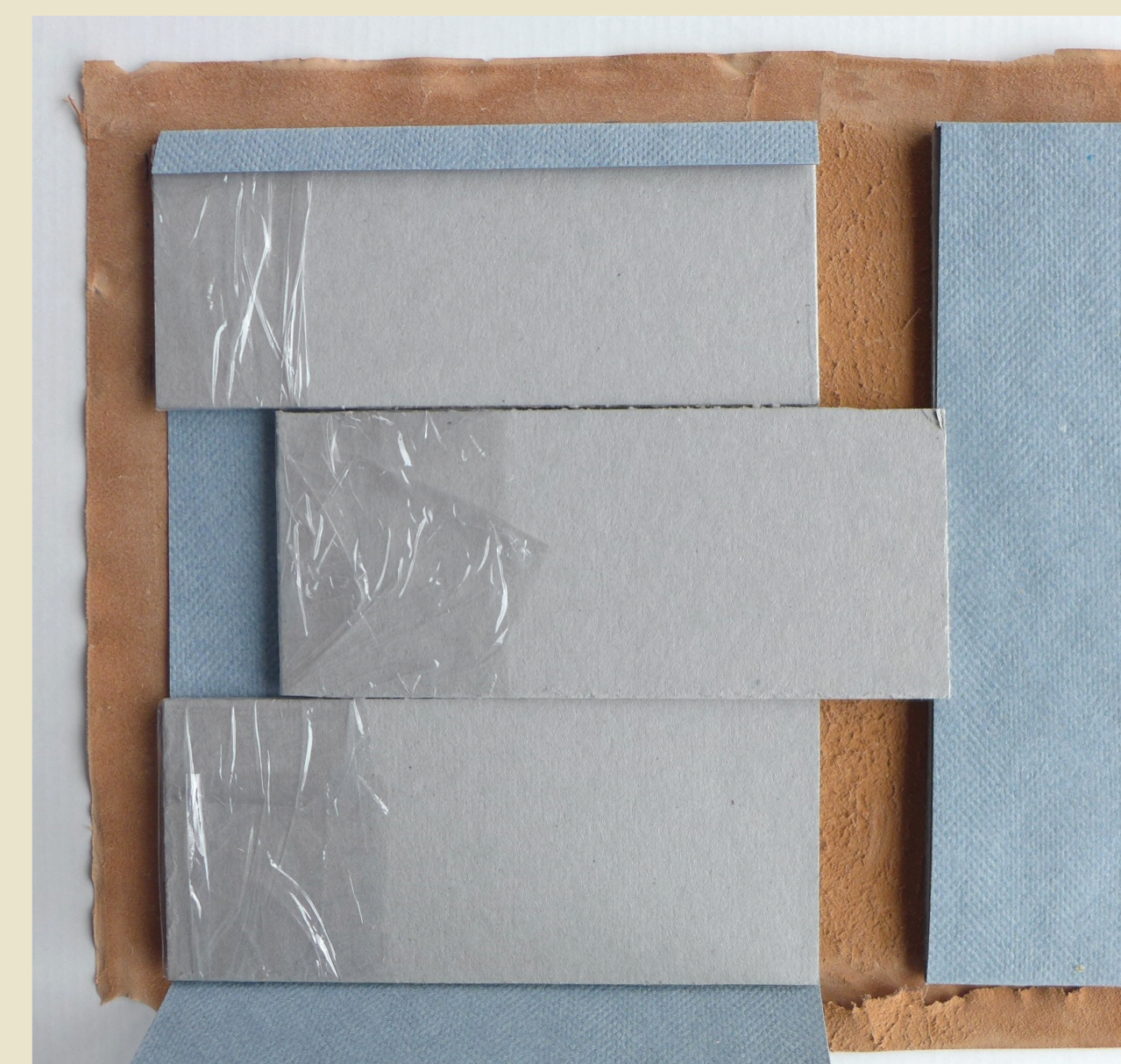
11. 3mm cardboard forming the mould is cut in 3 parts, the outer edges are covered with film.
