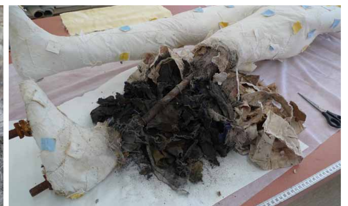
Fig. 5 The mildewed covering fabric had mouldered and needed to be replaced. Metal parts were corroding and in the heel of the foot the plaster had broken and was crumbling.
