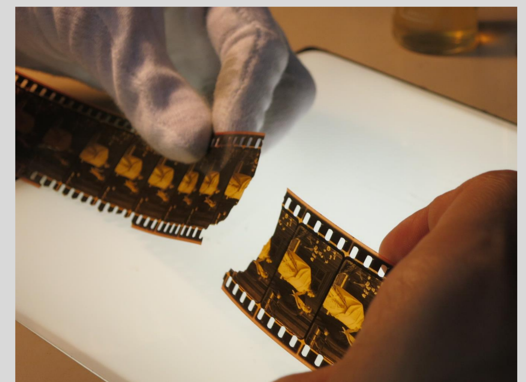
4. Reparation of tears and lacunas located at the perforation. L'Immagine Ritrovata laboratory, photo: Kadi Sikka, 2016
