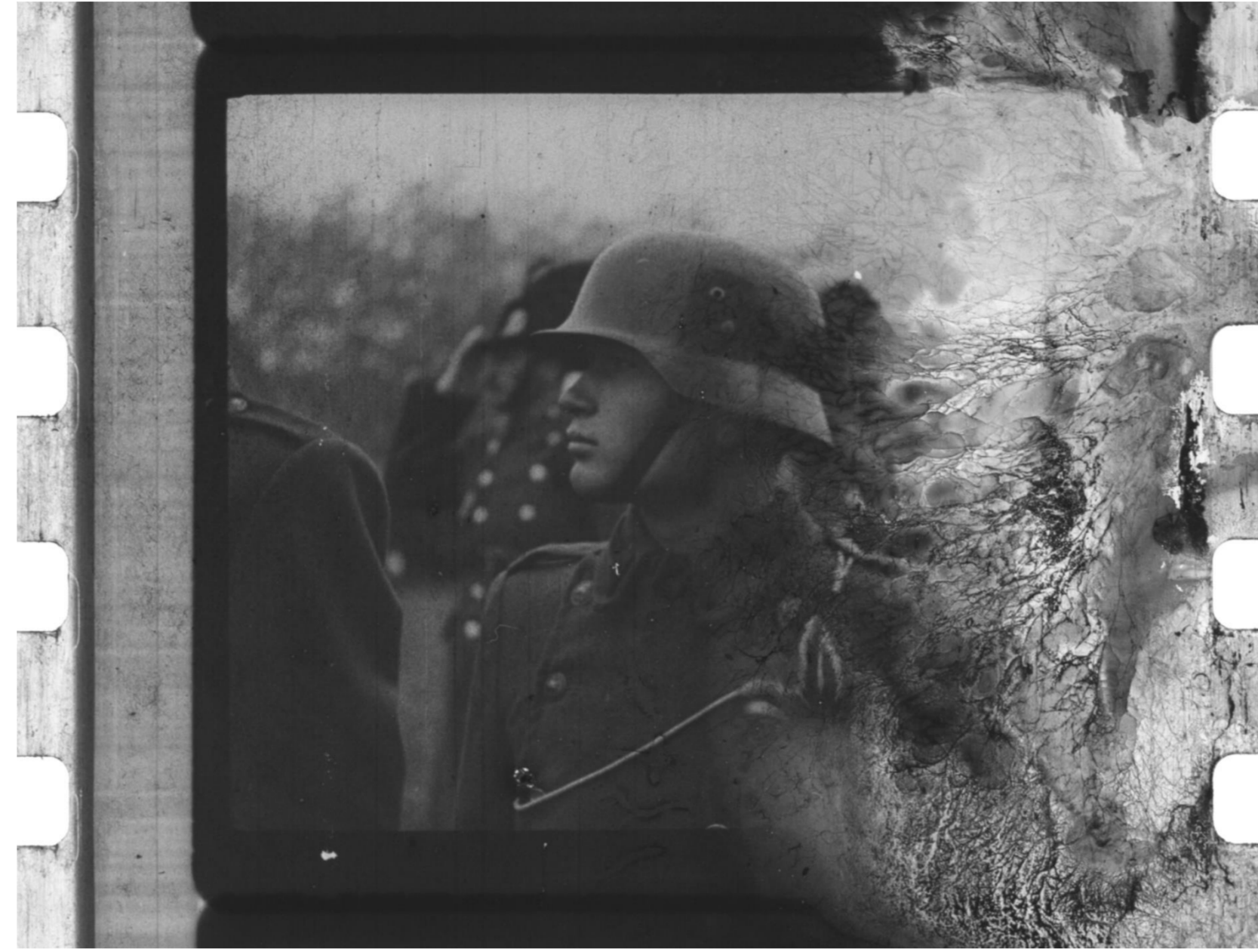
1. Decomposition of nitrate. UFA newsreel No. 535 (1942). 35mm b/w nitrate positive, EFA f 458 P-2793
